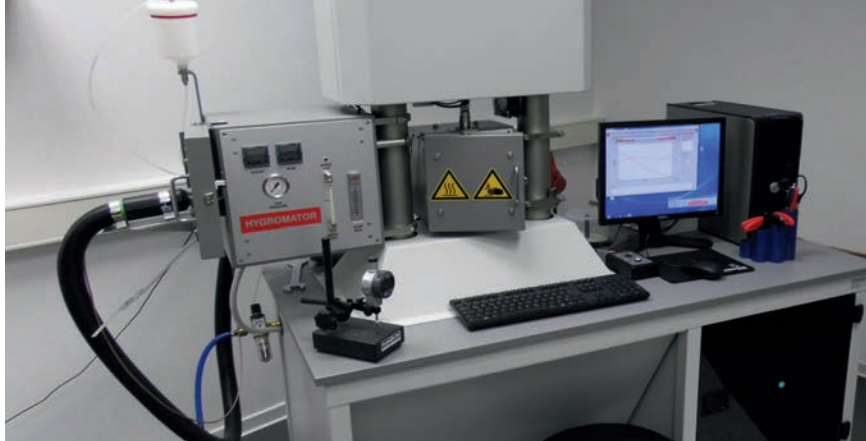
Prüfsystem Eplexor 500N (Gabo) incl. Hygromator/ Test system Eplexor 500N (Gabo) with Hygromator
