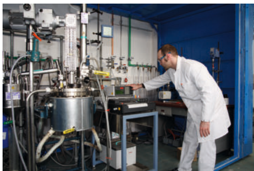
Autoklav zur Synthese/ autoclave for synthesis
